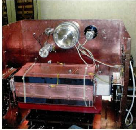
Fig. 2. The ferrite-core water-cooled RF-dipole, with a transverse RF magnetic-field integral of 1.5 Tmm peak-to-peak.
