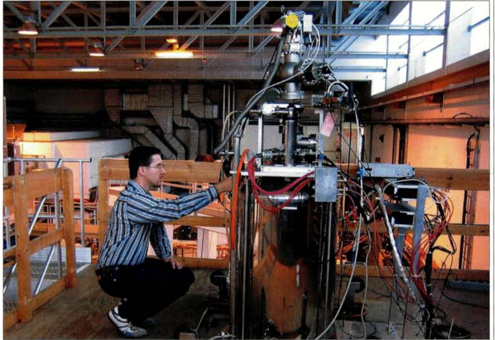
The ISOLTRAP Penning trap spectrometer at CERN's online isotope separator, ISOLDE, is providing precision mass measurements. (Photo: Alban Kellerbauer.)
