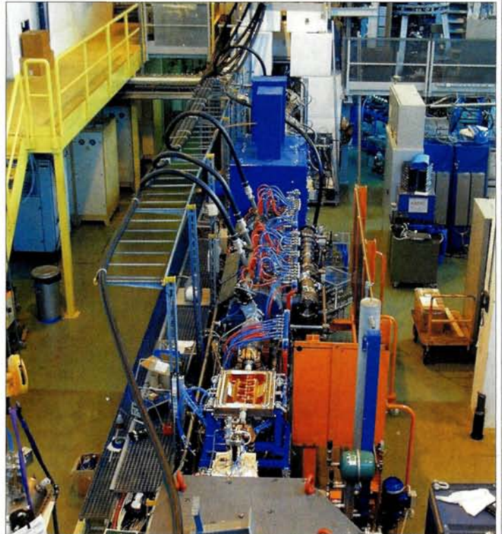
In this view of the REX-ISOLDE system, the last nine-gap resonator of the linear accelerator is clearly visible, open. In the background is the large Faraday cage containing the Electron Beam Ion Source (EBIS) on top of the REX trap.
