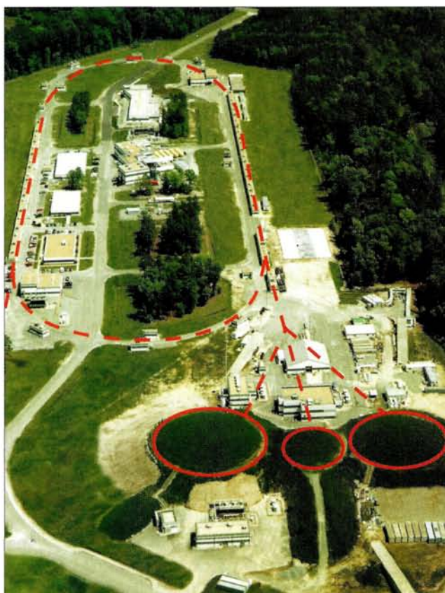
In this aerial photograph of the Continuous Electron Beam Accelerator Facility (CEBAF), the dashed line indicates the location of the accelerator and the circles indicate the positions of the three existing experimental halls.
